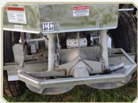
Lanco's Fertilizer Spreaders ground drive system includes a stainless steel, "positive" chain drive requiring less maintenance.
